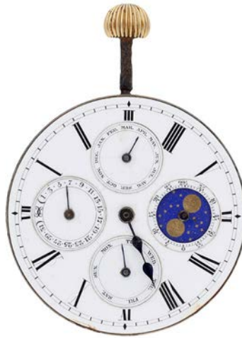
A REPEATER MOVEMENT WITH MOONPHASE DIAL, UNCASED, BY T. MARTIN & CO, LONDON, the white enamel dial with black Roman numerals and four subsidiary dials for month, date, day and seconds and moonphase, the movement with two chimes signed 'T. Martin & Co, 151 Regent Street, London, W.' and numbered '3739' (damaged), diameter 45mm. £100-£200
